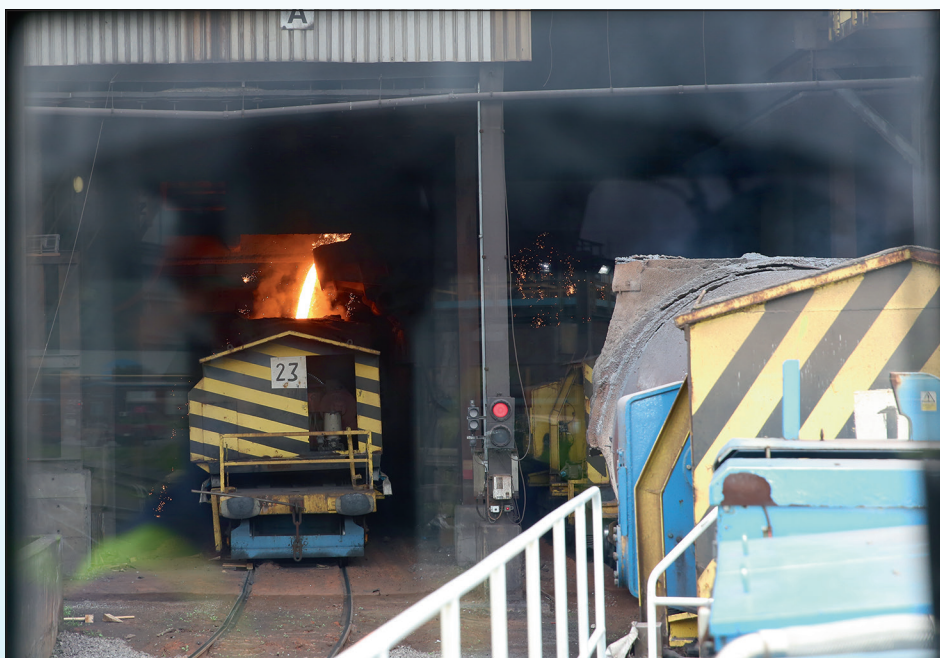
Above: A torpedo wagon is loaded with molten iron at blast furnace No. 5 before being taken to BOS plant.
