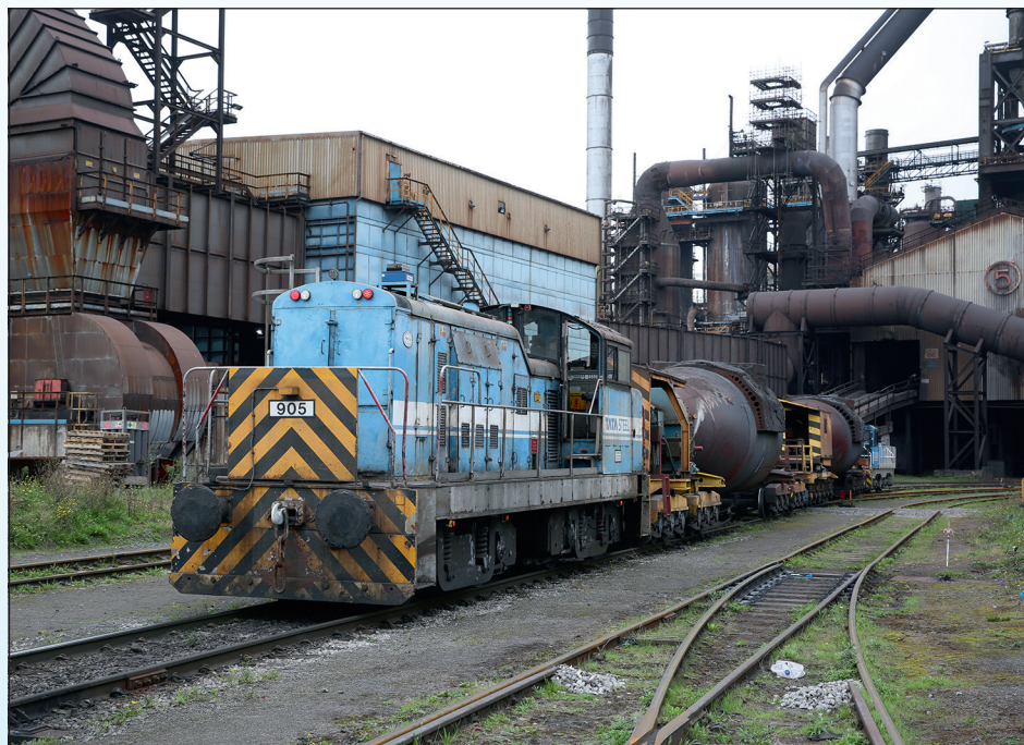
Above: One of the oldest locomotives in its original condition that is still in use, 1957-built 905 top-and-tails a train of torpedoes for blast furnace No. 5 with new Clayton CBD90 931.
