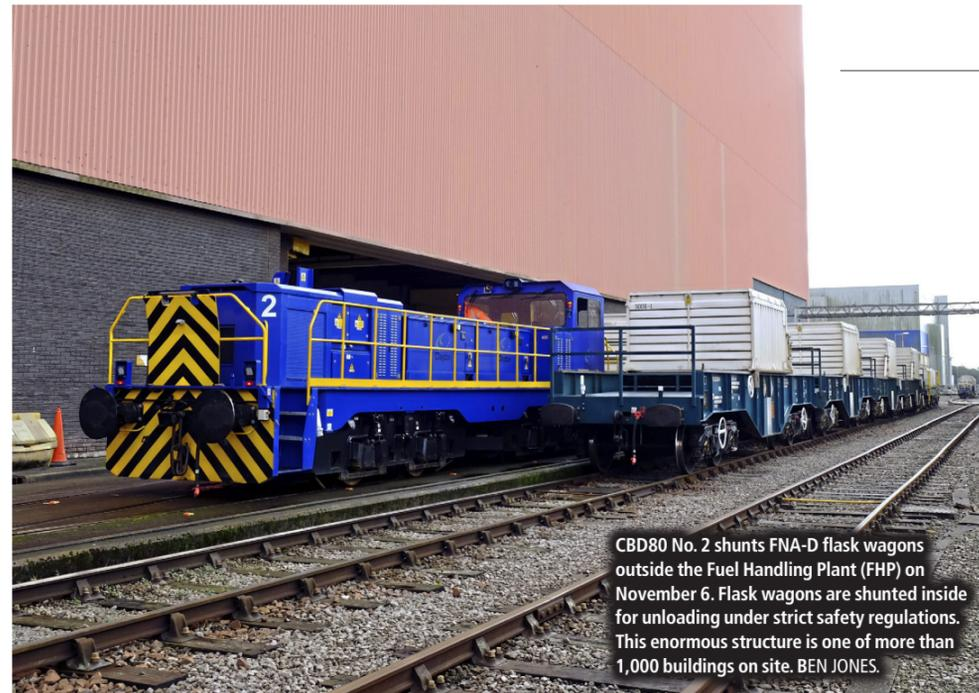
CBD80 No. 2 shunts FNA-D flask wagons outside the Fuel Handling Plant (FHP) on November 6. Flask wagons are shunted inside for unloading under strict safety regulations. This enormous structure is one of more than 1,000 buildings on site. BEN JONES.
