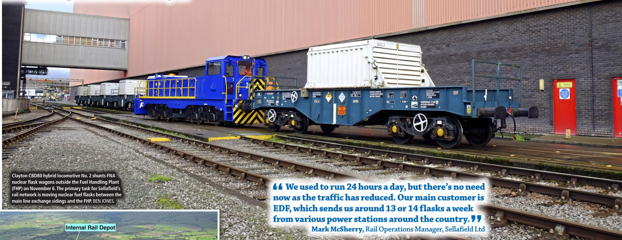
Clayton CBD80 hybrid locomotive No. 2 shunts FNA nuclear flask wagons outside the Fuel Handling Plant (FHP) on November 6. The primary task for Sellafield's rail network is moving nuclear fuel flasks between the main line exchange sidings and the FHP. BEN JONES.
