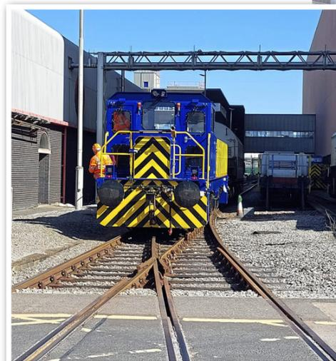
Above: The internal rail network operates a strict safety regime, with three operating zones. When a train enters a zone, all road traffic is halted at crossings and only one train is permitted to move in each zone. MARK MCSHERRY.
