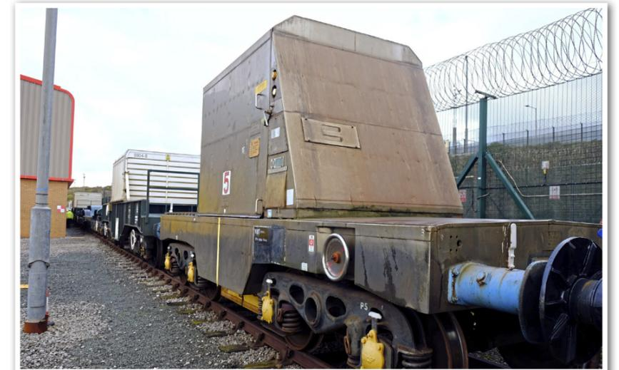
The plant's rarely seen fleet of specialist internal wagons includes multi-purpose 'skeleton' wagons and stainless steel-clad vehicles for moving nuclear fuel flasks. Now limited to moving empty flasks for storage, wagon 5 stands with an FNA-D at Sellafield DRS depot on November 6. BEN JONES.
