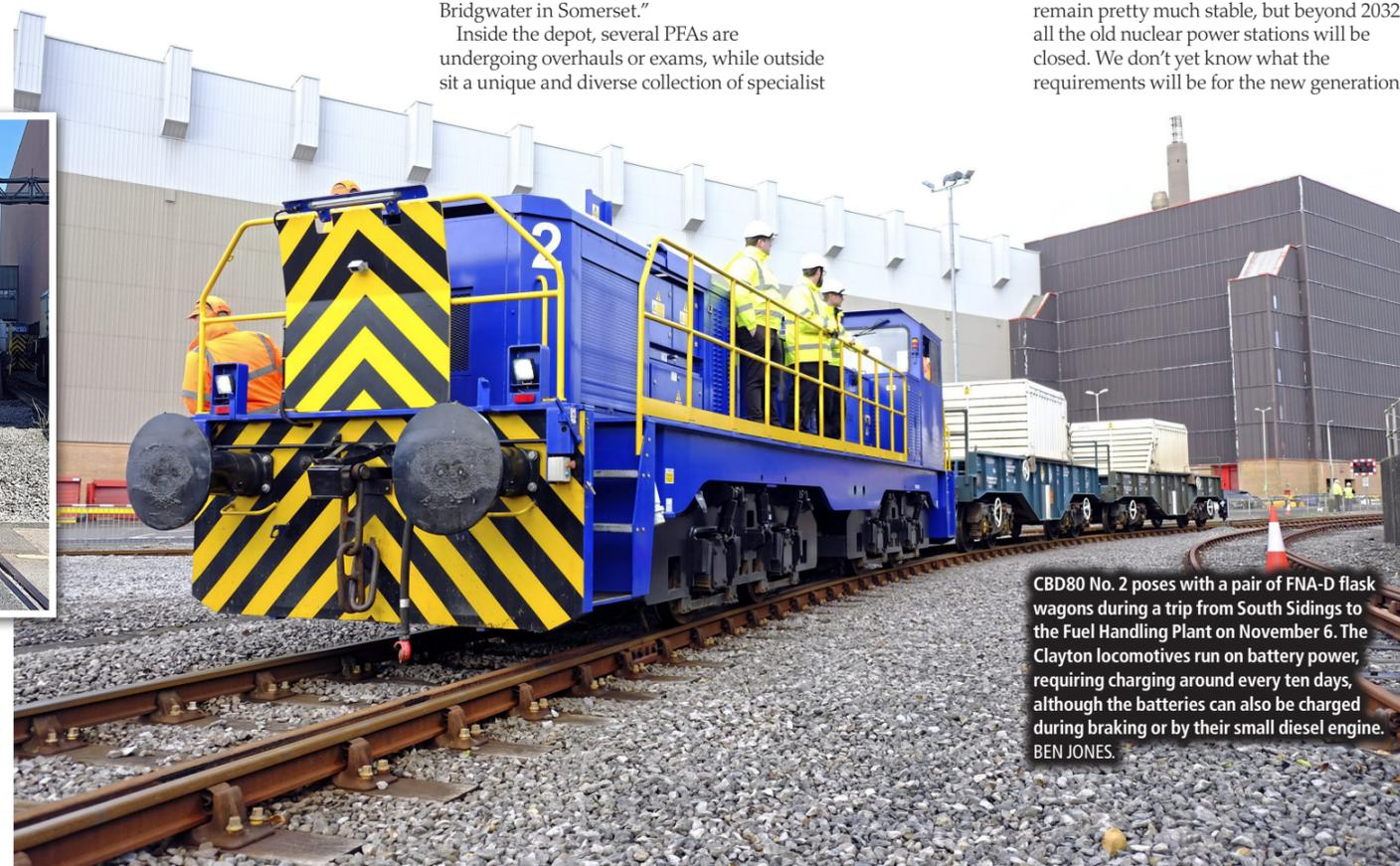
CBD80 No. 2 poses with a pair of FNA-D flask wagons during a trip from South Sidings to the Fuel Handling Plant on November 6. The Clayton locomotives run on battery power, requiring charging around every ten days, although the batteries can also be charged during braking or by their small diesel engine. BEN JONES.
